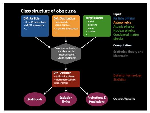
This high level of modularity in this type of calculation needs to be reflected in the code's polymorphic structure. The goal of *obscura* is to provide for each of the different inputs one generic interface or abstract base class, that comprises the general required functionalities, without specifying the detailed implementations further. These depend on a multitude of assumptions which can change in different projects, for different users, etc.
